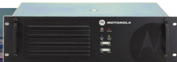
Left: TCIT's huge seaport in Vietnam covers a total area of 40 hectares featuring three berths, 29 cranes, 56 tractors and four reach stackers. Its MOTOTRBO Capacity Plus comms system from Motorola Solutions is based around four R8200 repeater units (above).
