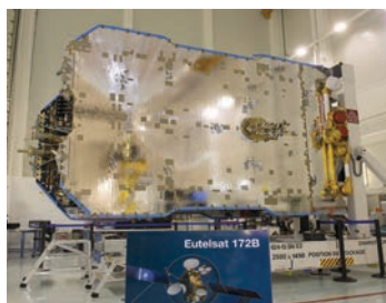
EUTELSAT 172B has been built with innovative features such as the flexibility to dynamically distribute beam power, robotic arms for orbital control, and parts made using 3D-printing. PHOTO: AIRBUS SPACE & DEFENCE.
