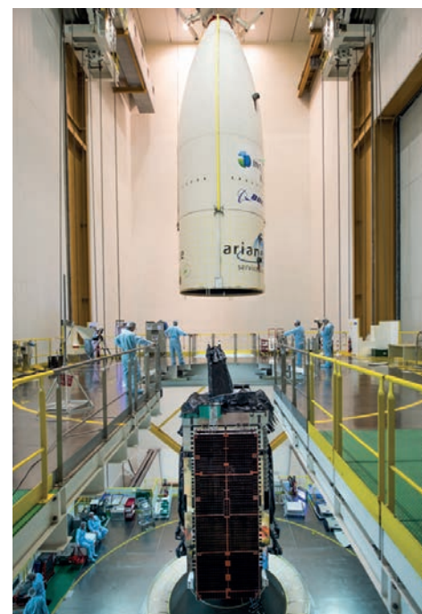
The payload fairing being positioned over Intelsat 29e which is integrated to the top of an Ariane 5 launcher. It went on to a successful launch on 27 January 2016, and is the first of Intelsat's satellites to use the revolutionary EpicNG HTS platform.
