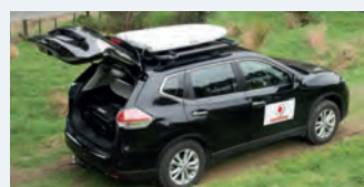
The Z-Car has a 4G small cell built into its boot which provides mobile coverage even in motion.
