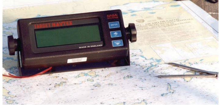
Navtex is a navigational system used on board the vessels to provide short range maritime safety information on coastal waters
