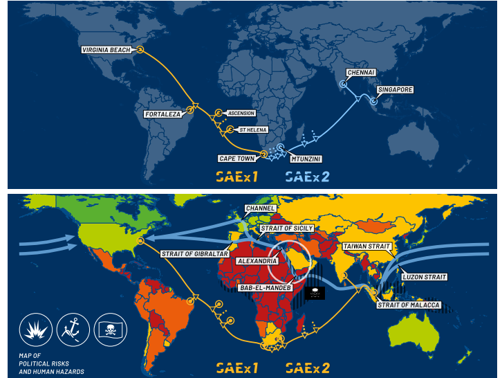
Top: the new project will first cross the Atlantic linking Cape Town to the US via Brazil, and then extend across the Indian Ocean in phase two. Bottom: the cable aims to avoid potentially unstable areas.
