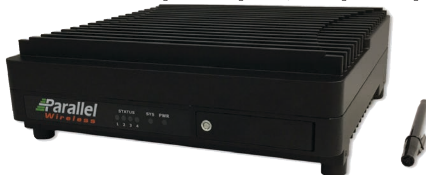
Parallel Wireless Converged Wireless System can act as a small cell in a hetnet system and can be used in vehicles to support 'Bring Your Own Coverage' capabilities.
