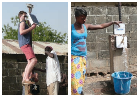
Left: eWATER's solar powered smart tap fully integrates mobile money, IoT and NFC technologies. Right: the tap dispenses clean fresh water after reading a user's pre-paid eWATER NFC tag.
