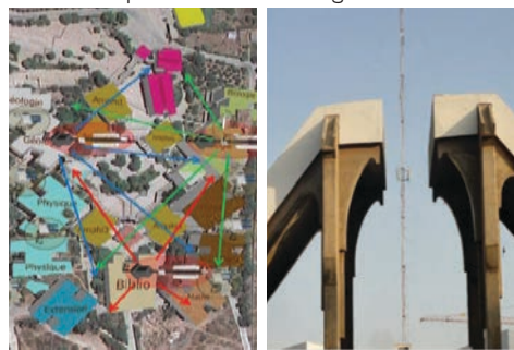
Left: Altai's partner in Morocco carried out a site survey of the university and discovered several challenges. Right: the infrastructure includes APs installed on light poles to provide wide area Wi-Fi coverage as well as radios to extend signals to indoor areas.
