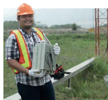
DAMM's TetraFlex outdoor base station is optimised for direct installation in harsh environments and has an IP65 enclosure.
