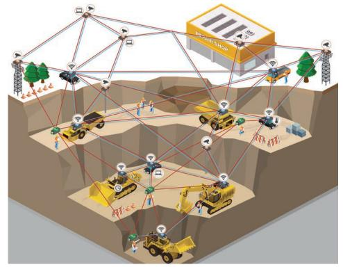
A kinetic mesh network topology features multiple nodes that basically act as transportable mini cell towers. Virtually anything in the organisation's infrastructure can be turned into networking equipment. Giving the network the ability of 'wheels' means that even outer-edge communications would be completely reliable and provide a previously impossible connection directly to a control centre.
