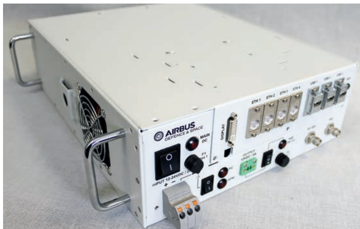
Left: Airbus Defence and Space's standalone Tactilon Cell can be used to create a small LTE network. It comprises a base station, terminals, LTE software and an app server for mission-specific apps. All the cell's features comply with 3GPP standards. Right: the recently launched Dabat integrates a complete TETRA radio and smartphone in one device. Airbus says it can work on any TETRA network.
